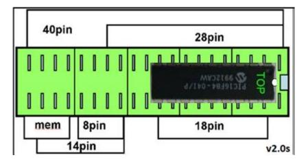
The notch on the device should always points towards TOP (handle of the ZIF socket). There are marks on the board to assist you with placing devices correctly in the socket.
