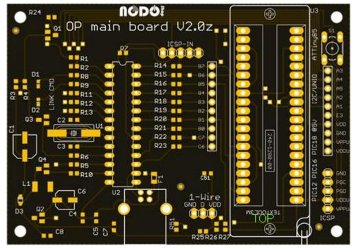
This kit is based on <u>http://openprog.altervista.org/</u> which handles PICs up to 20 pin and EEproms and can program additional devices using plug in extension boards (not supplied). Surface mount components have been used to ease assembly and reduce costs, as well as a ZIF socket for long life and convenient operation. This manual should be read together with the website which gives a lot more information on the design.
