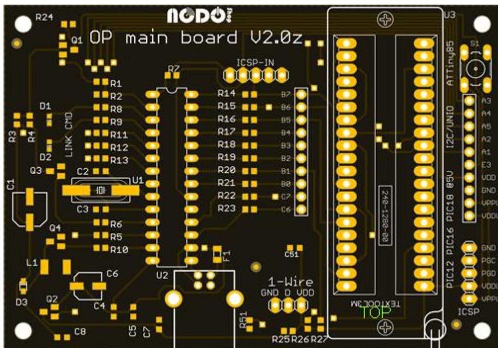
This kit is based on <http://openprog.altervista.org/> which handles PICs up to 20 pin and EEproms and can program additional devices using plug in extension boards (not supplied). Surface mount components have been used to ease assembly and reduce costs, as well as a ZIF socket for long life and convenient operation. This manual should be read together with the website which gives a lot more information on the design.
