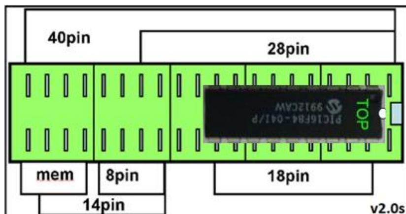
The notch on the device should always point towards TOP (handle of the ZIF socket). There are marks on the board to assist you with placing devices correctly in the socket.
